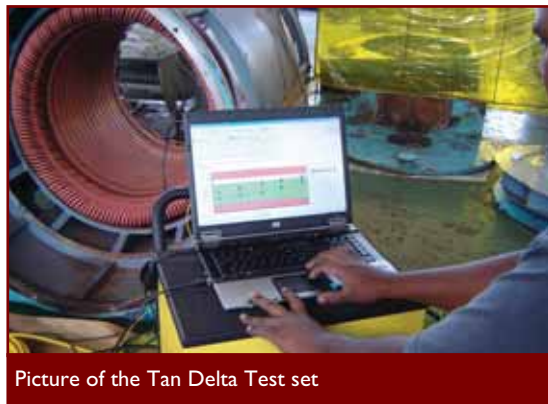
A service engineer is pictured performing a tan delta test
